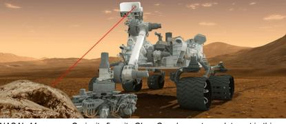
impossible — in the middle of a long drive, NASA's Mars rover Curiosity fires its ChemCam laser at a rock target in this perhaps, or when the schedules of Earth, Mars artist's illustration. ChemCam has fired more than 350,000 shots on Mars as and spacecraft activities lead to delays in of July 2016. Credit: NASA/JPL-Caltech sharing information between the planets,"
