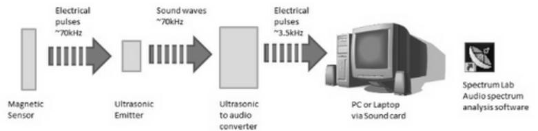
Figure 2: Schematic layout of magnetometer: Sensor to PC
